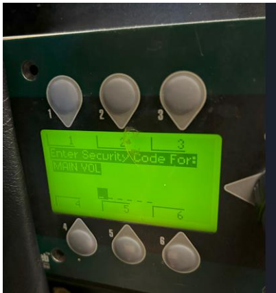
Figure 14 - Venue sound system management panel. Password protected. A bass reduction of -40dB was applied to achieve 90A/100C under these conditions in the venue.
