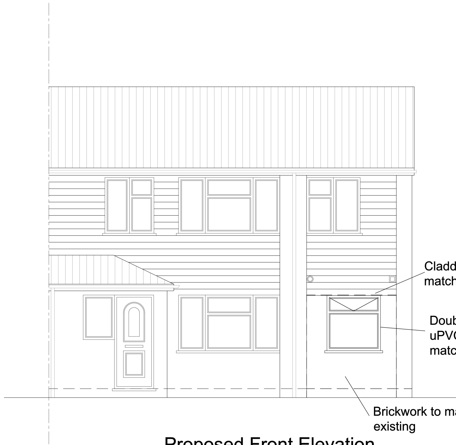
Proposed Front Elevation ⊙ Denotes existing gas boiler vent
