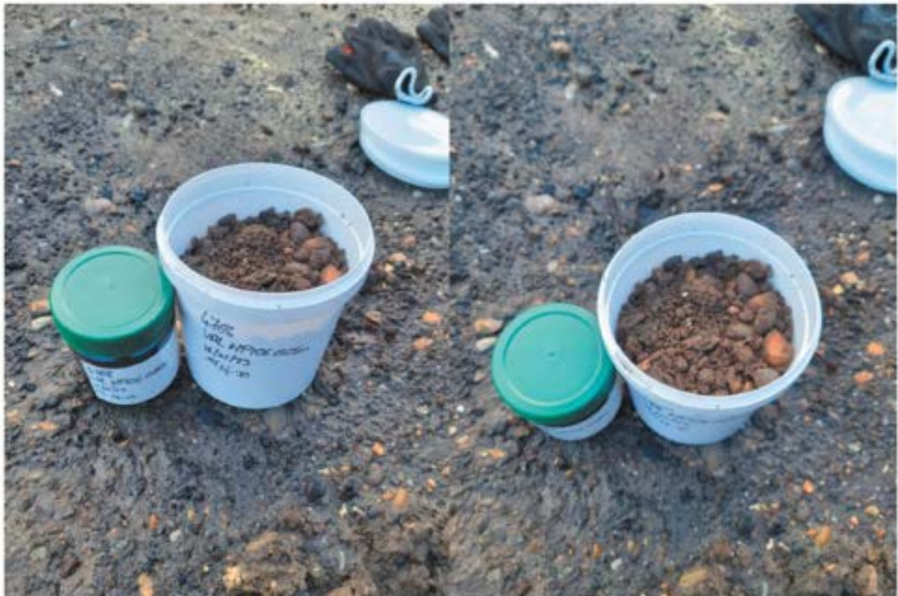
Photos 9 + 10 - Example soil validation samples from beneath the tarmac hardstanding
