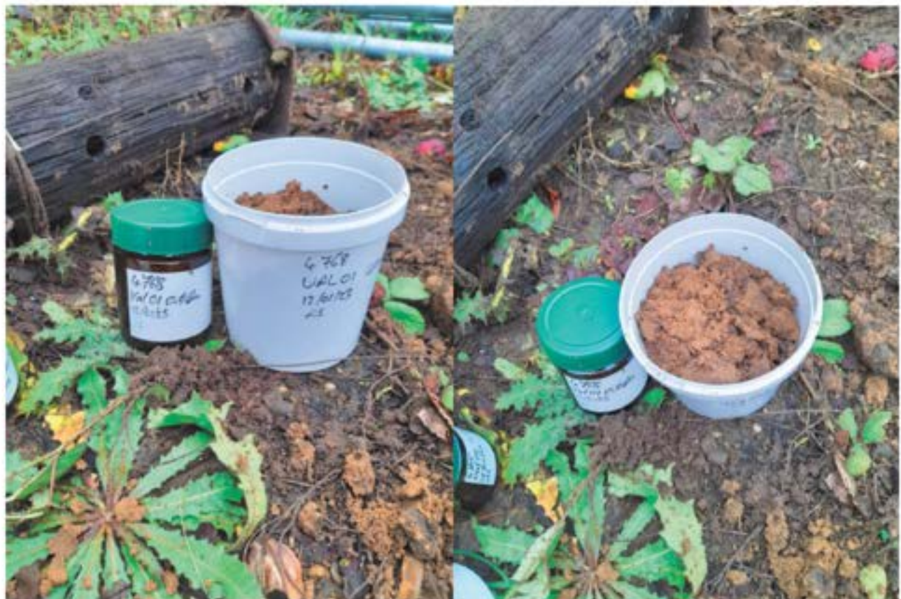
Photos 3 + 4 - Example soil validation sampling for testing
