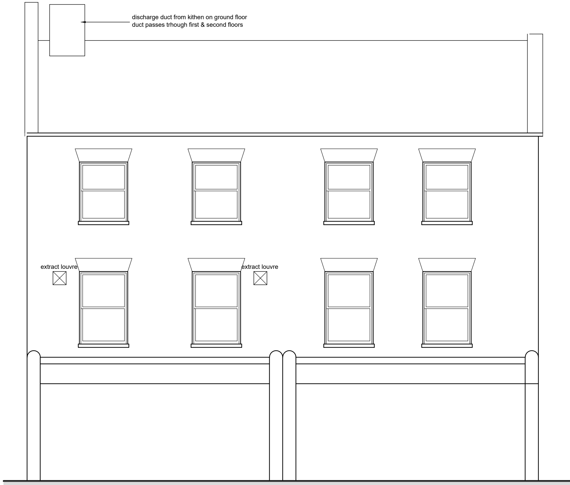
FRONT ELEVATION ON C-C AS EXISTING (1:50)
