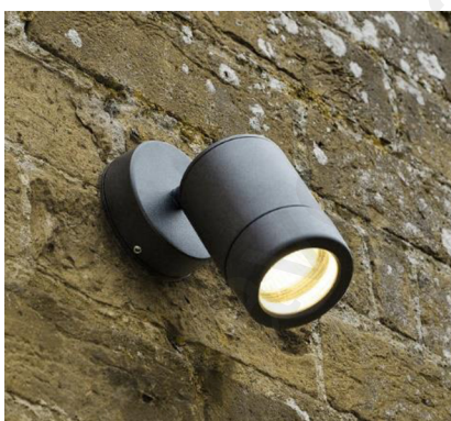
Single adjustable wall light powder coated aluminium, black 154mm H x 78mm W 4.5w warm white 2700K LED, 35° fitted near entrance doors & doors to garden
