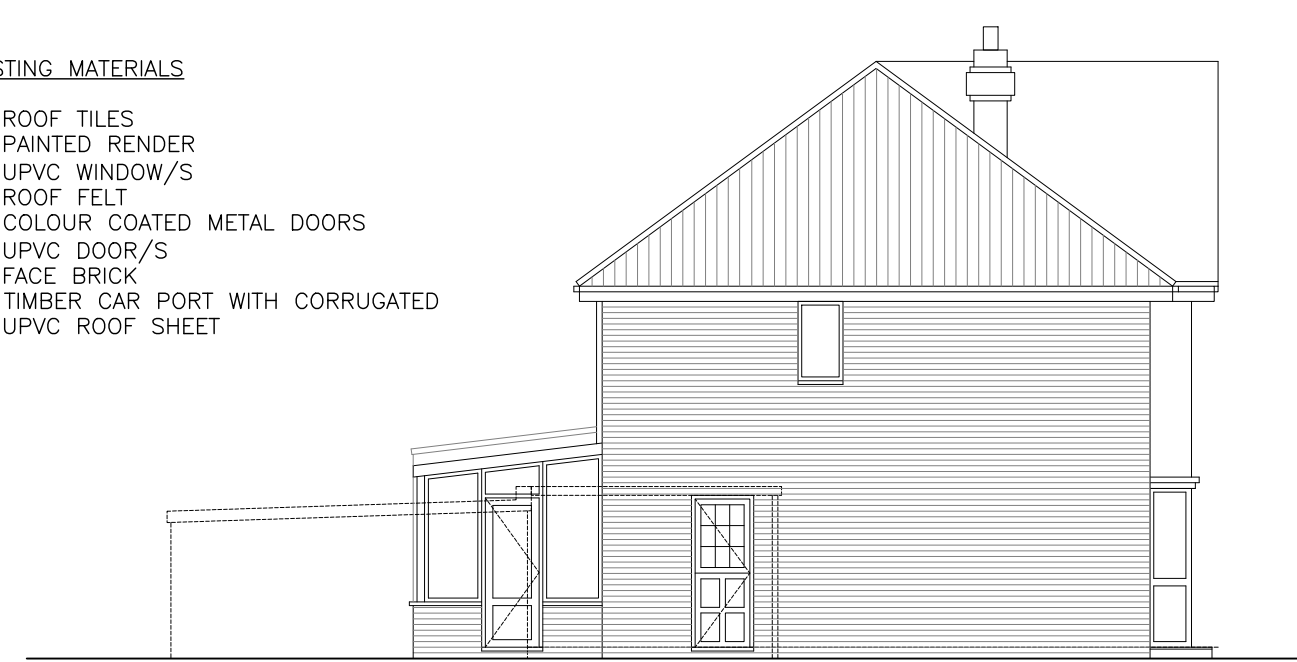
09 Existing Side Elevation
