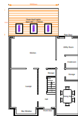
Proposed Extension Roof Plan Showing Roof Lights
