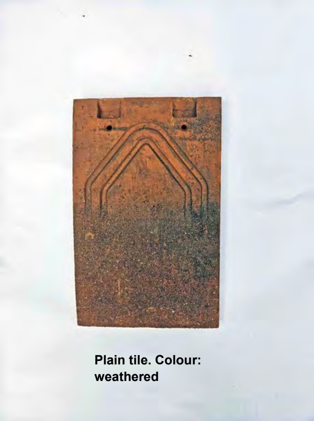
B1 & B6: Clay roof tiles
