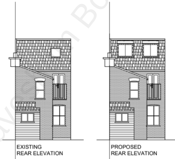
Rear Elevations Showing the Proposed Loft Dormers.
