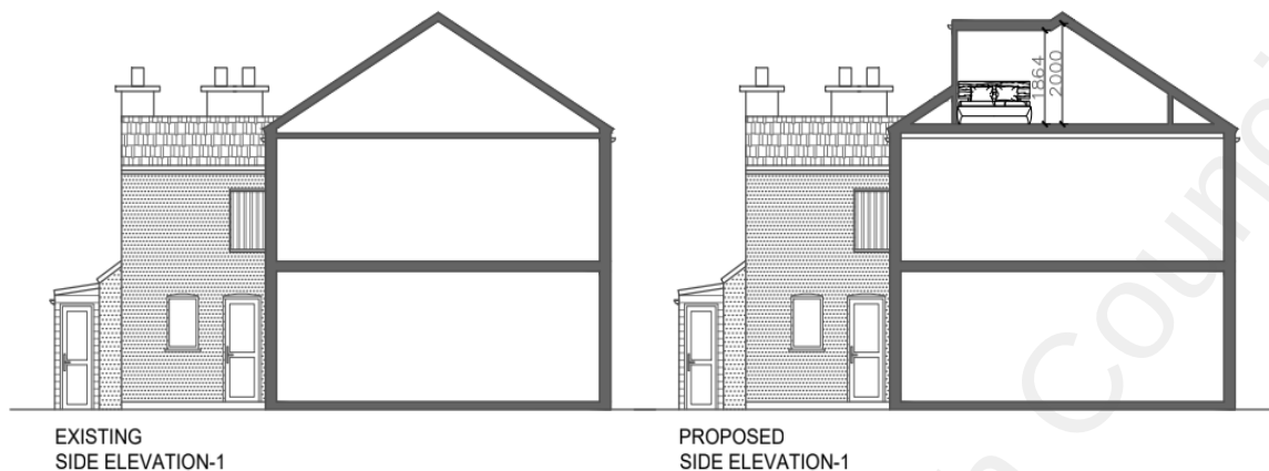
Side Elevation Plans Showing the Proposed Section plan and elevations for loft floor.
