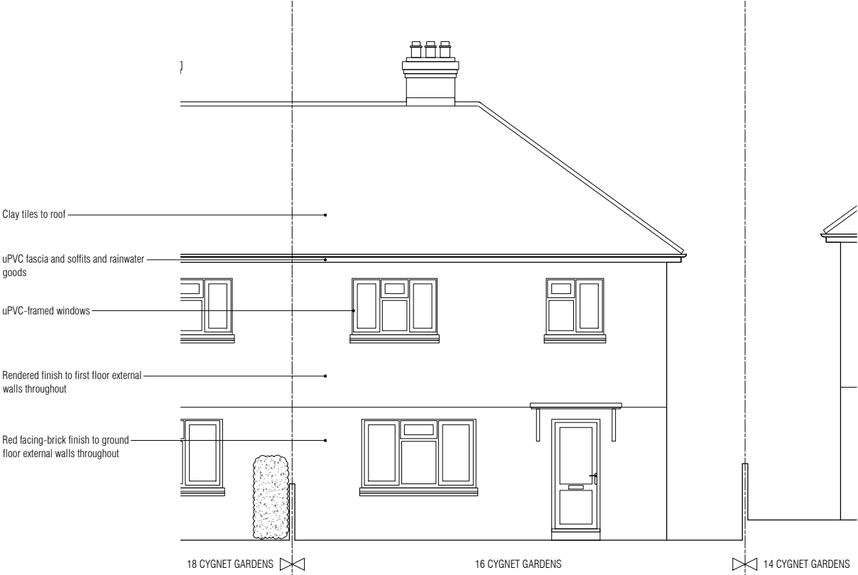
1. EXISTING FRONT ELEVATION
