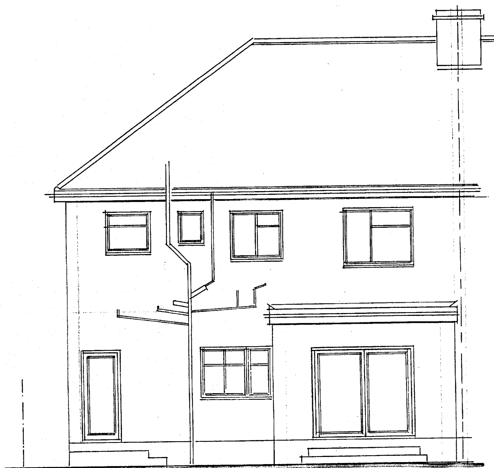
EXISTING REAR ELEVATION
