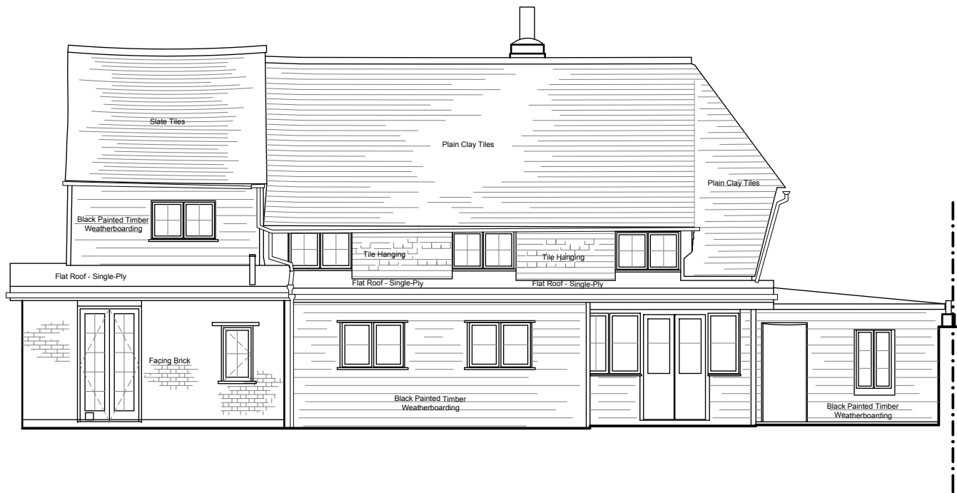
HOUSE EXISTING/PROPOSED SOUTH-WEST ELEVATION NO ALTERATIONS PROPOSED
