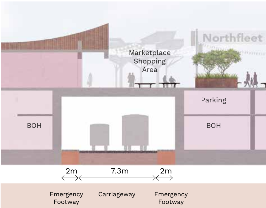
Typical section through the Marketplace podium tunnel
