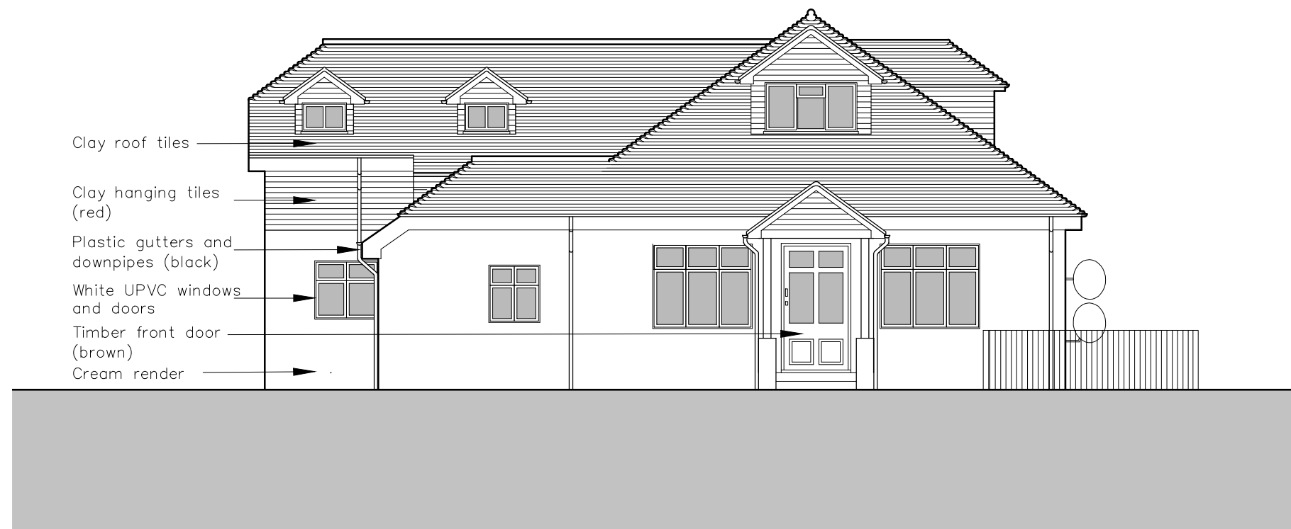
Existing Side (South-West) Elevation 1:100
