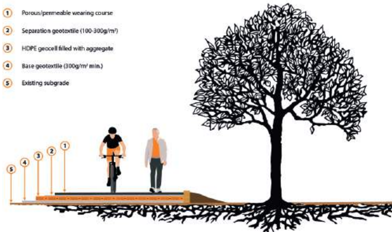
Figure 1: The basic approach to using cellular confinement systems for ground protection near trees [image courtesy of Core LP].
