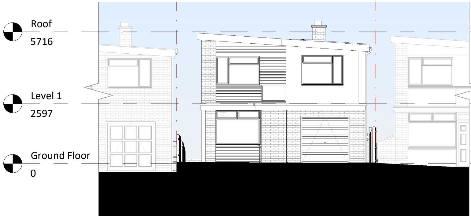
5 Existing Front Elevation 1 : 100
