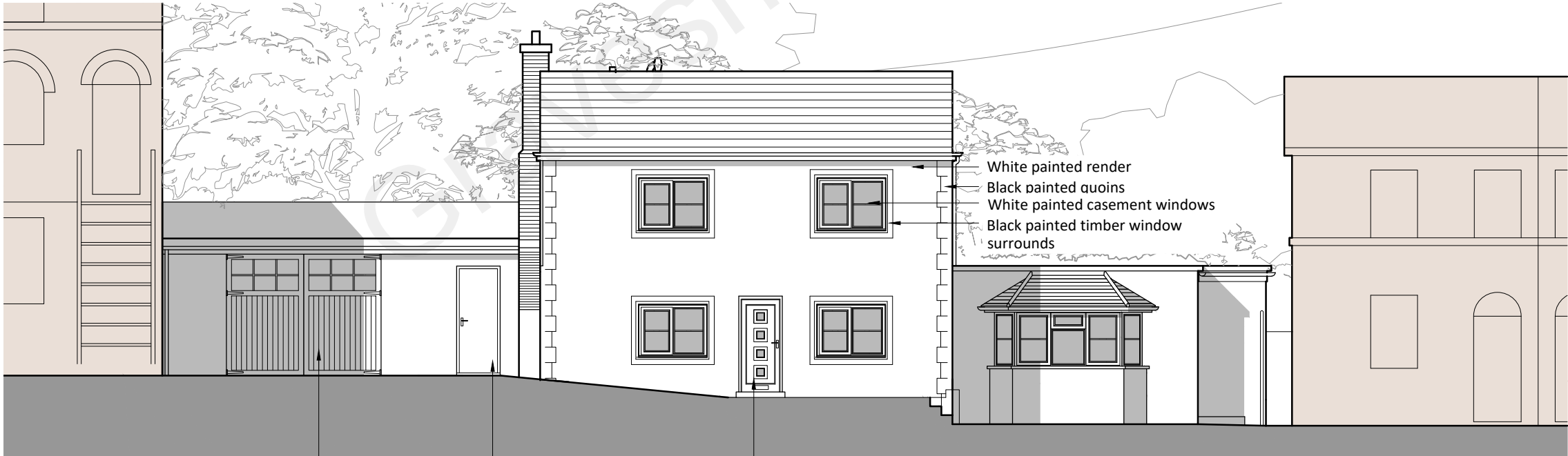
Proposed Front Elevation (South-East) 1:100
