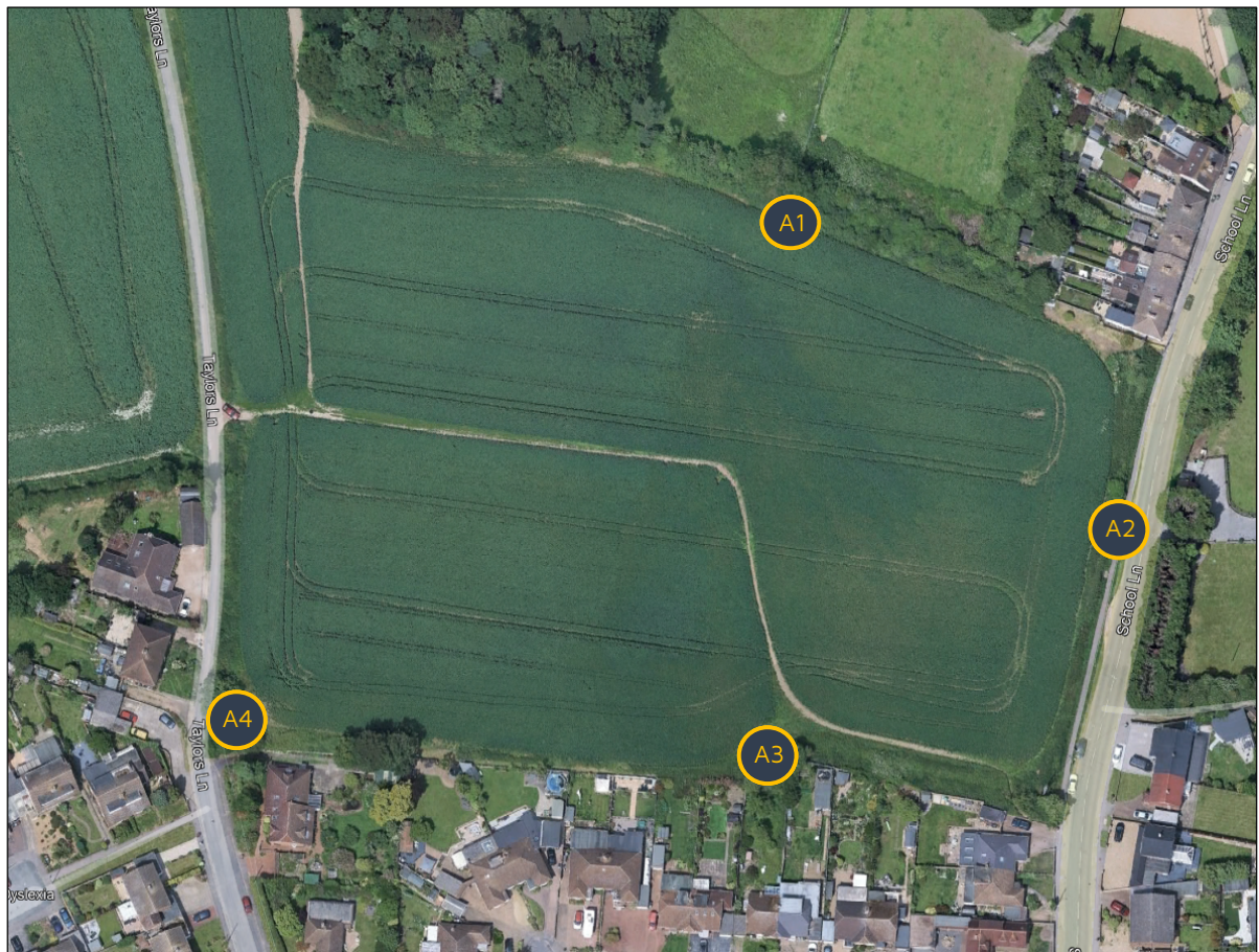
Figure 5.1: Noise Monitoring Locations
