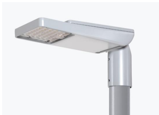
Figure 2.5.1 – luminaire used within the lighting calculation – column mounted at 6m, Holophane S-Line 24W, IP66, 3000K LED colour temperature, Type II Medium distribution
