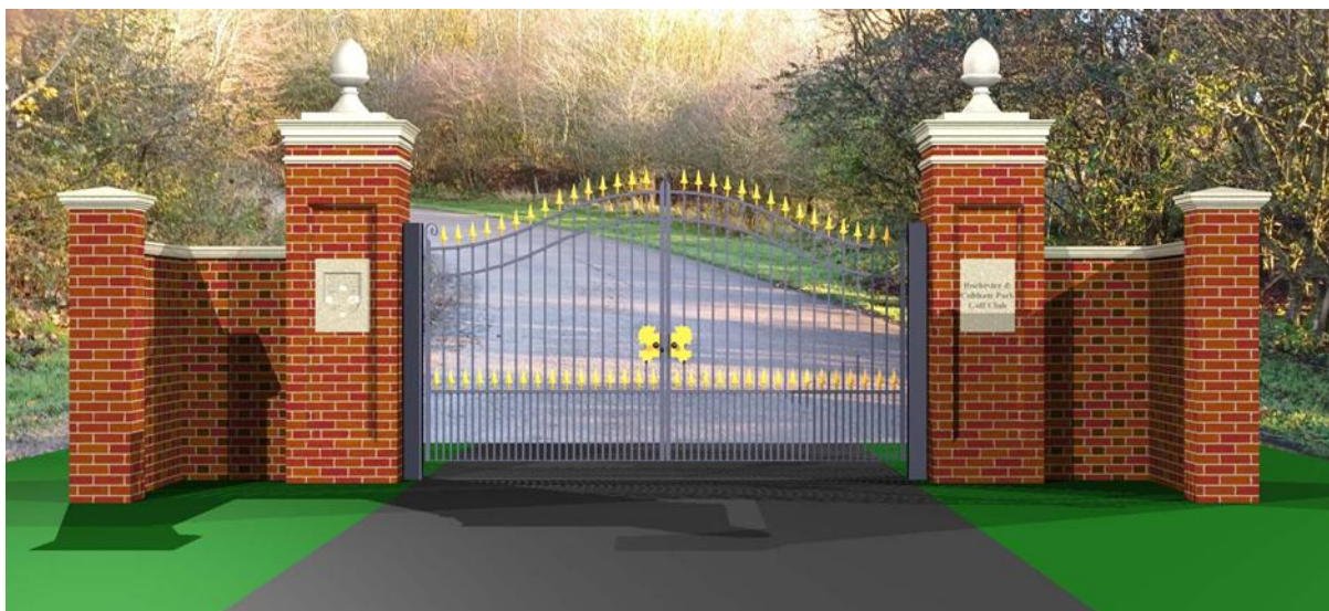
Figure 4: Proposed gate posts & wing walls
