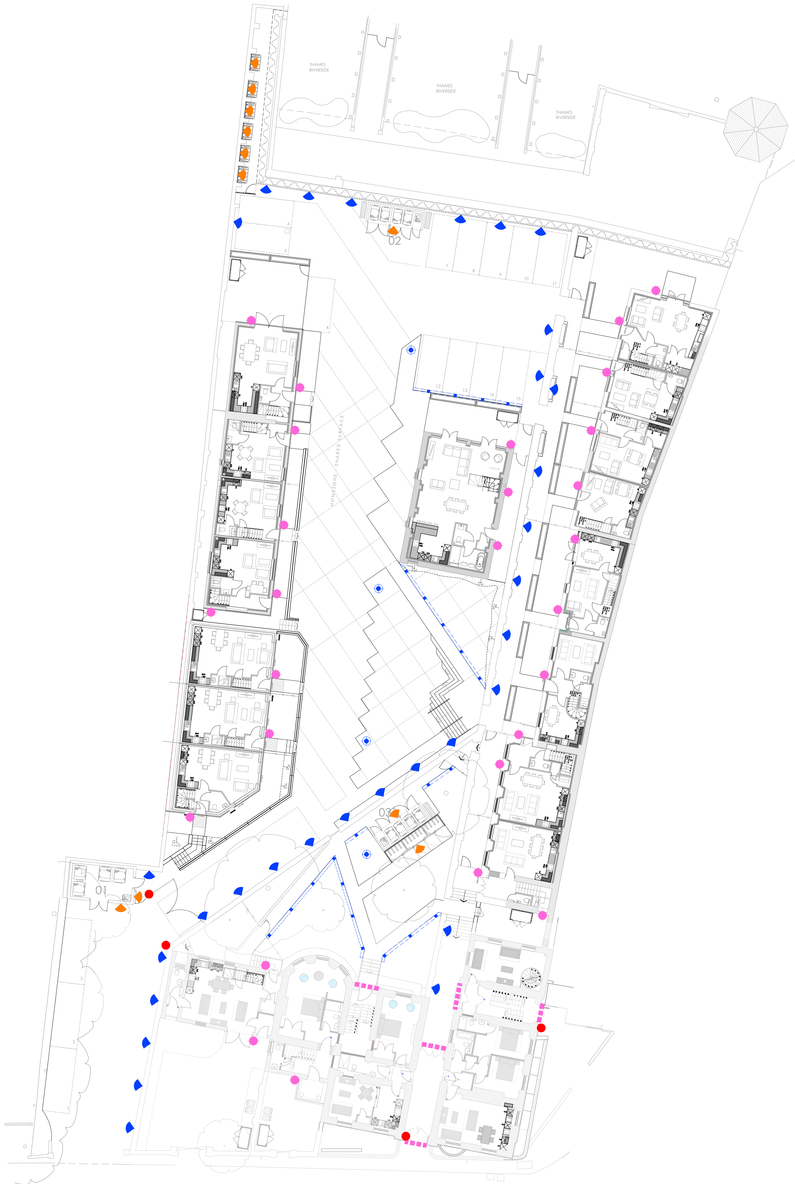
External Lighting and Access Control Intent Plan
