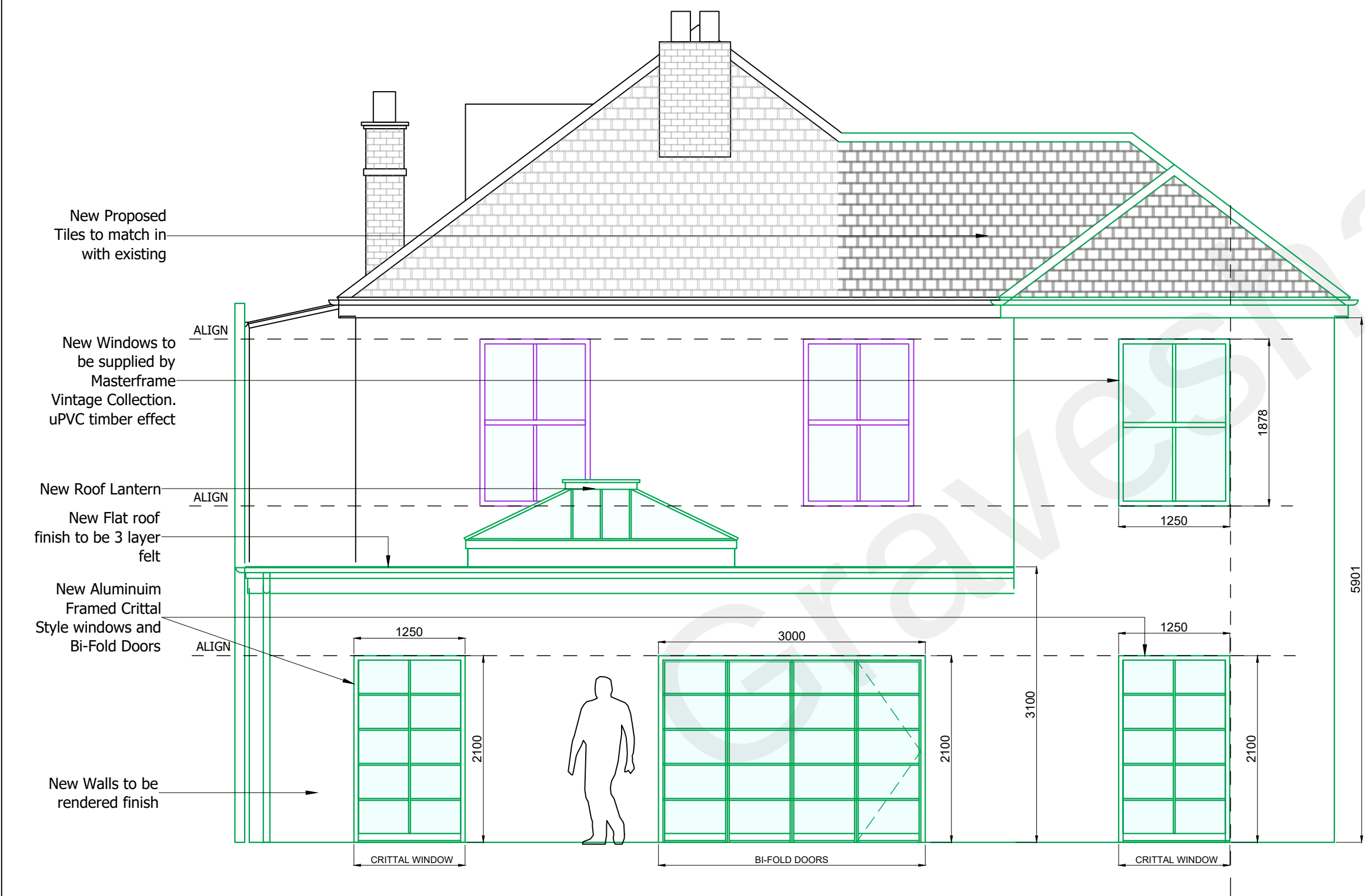
ELEVATION C: PROPOSED REAR ELEVATION SCALE 1:50@A1
