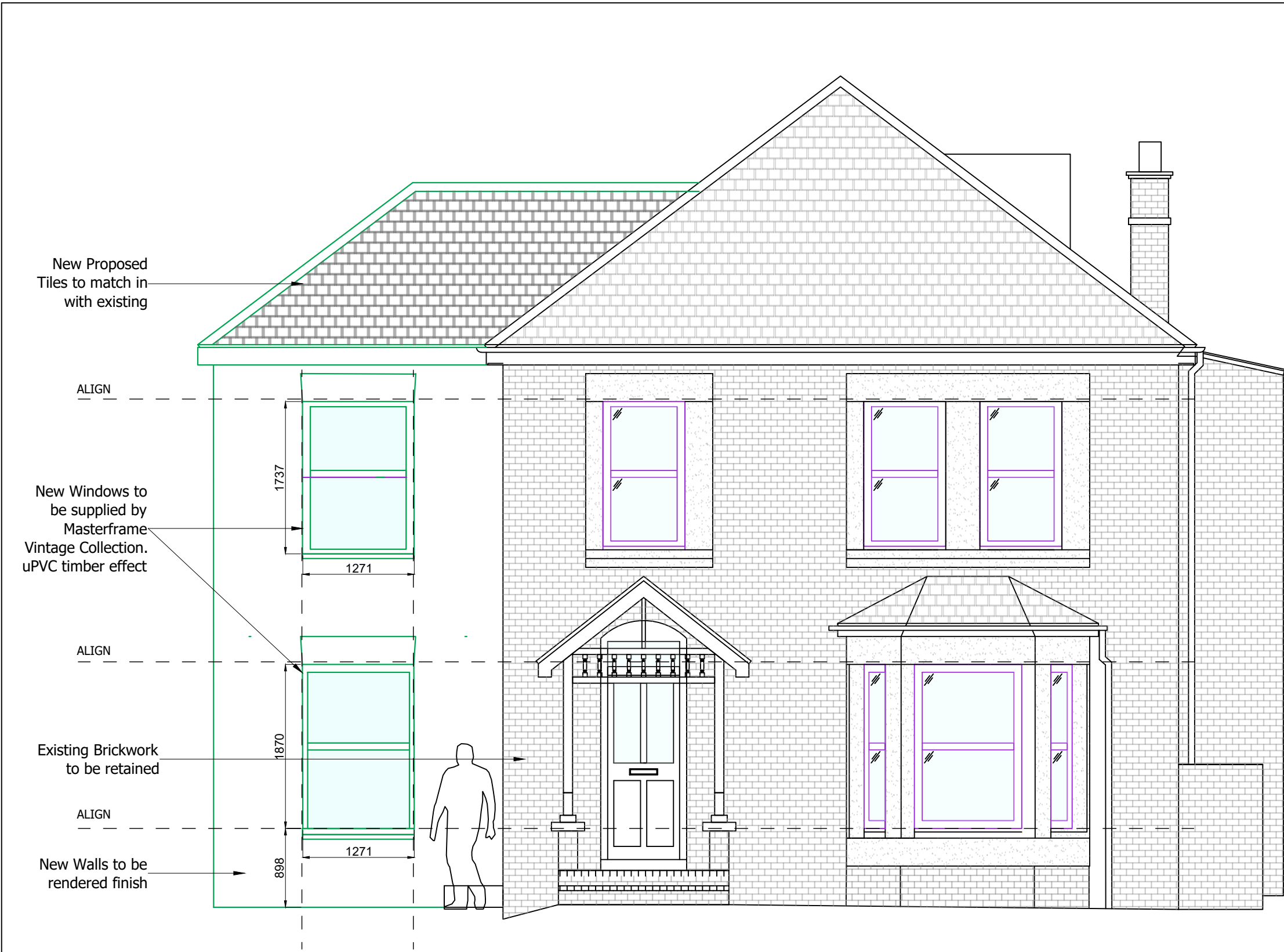
ELEVATION A: PROPOSED FRONT ELEVATION SCALE 1:50@A1
