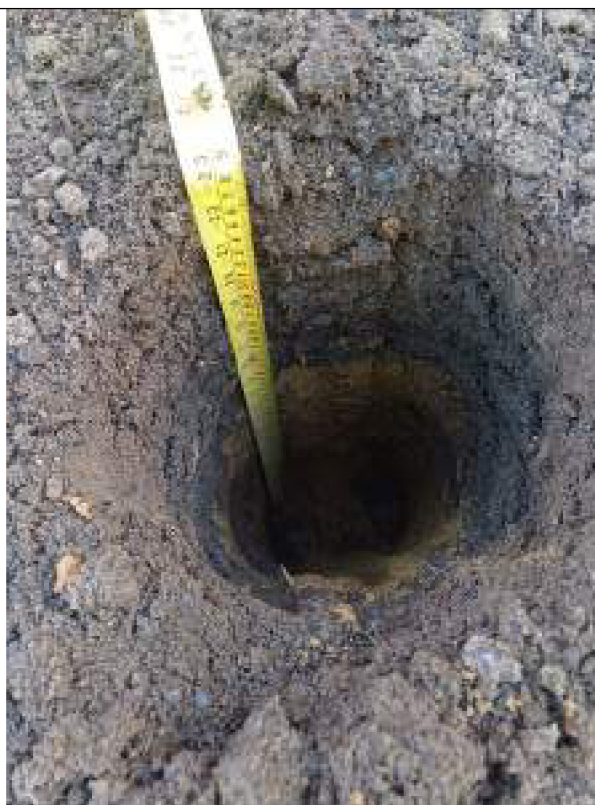
Plate 2: Plot 122 clean cover thickness
