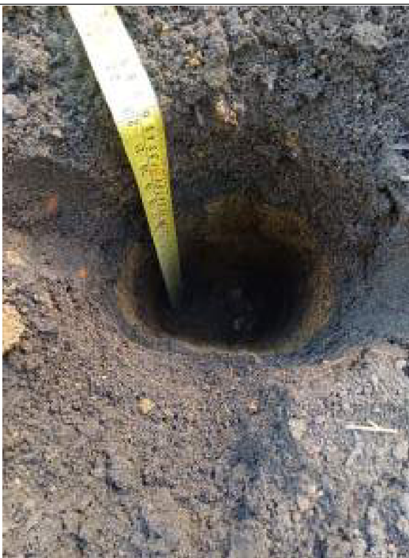
Plate 6: Plot 124 clean cover thickness
