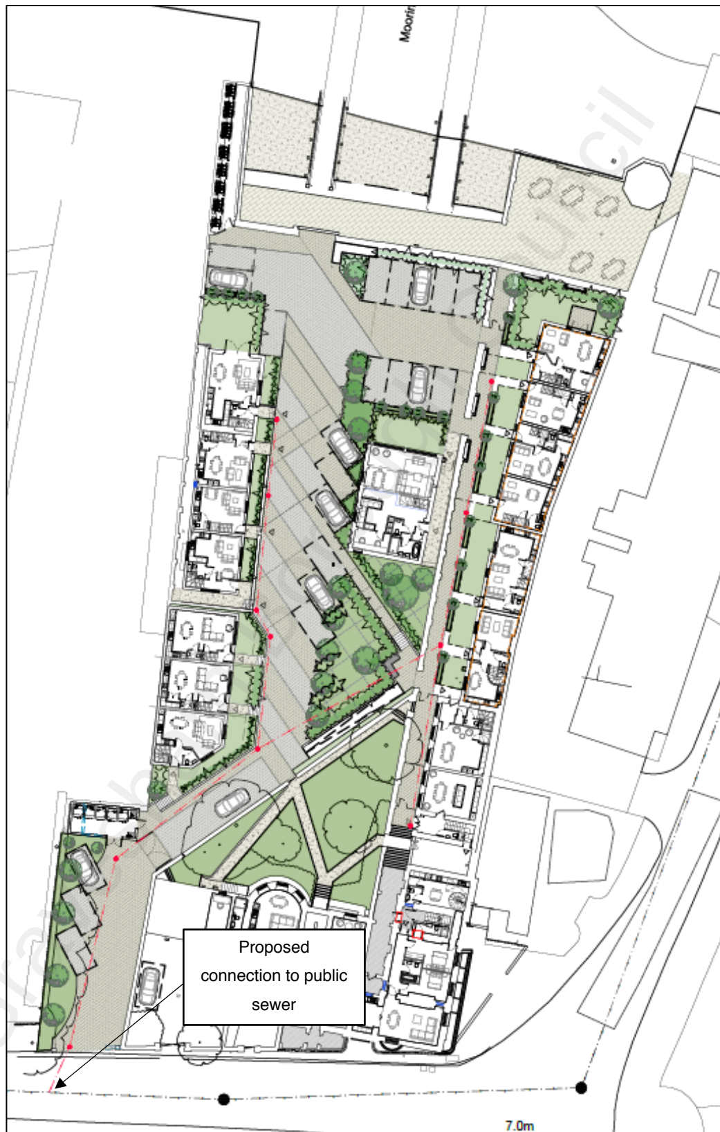
Figure 9.1 – Proposed connection to foul sewer network.
