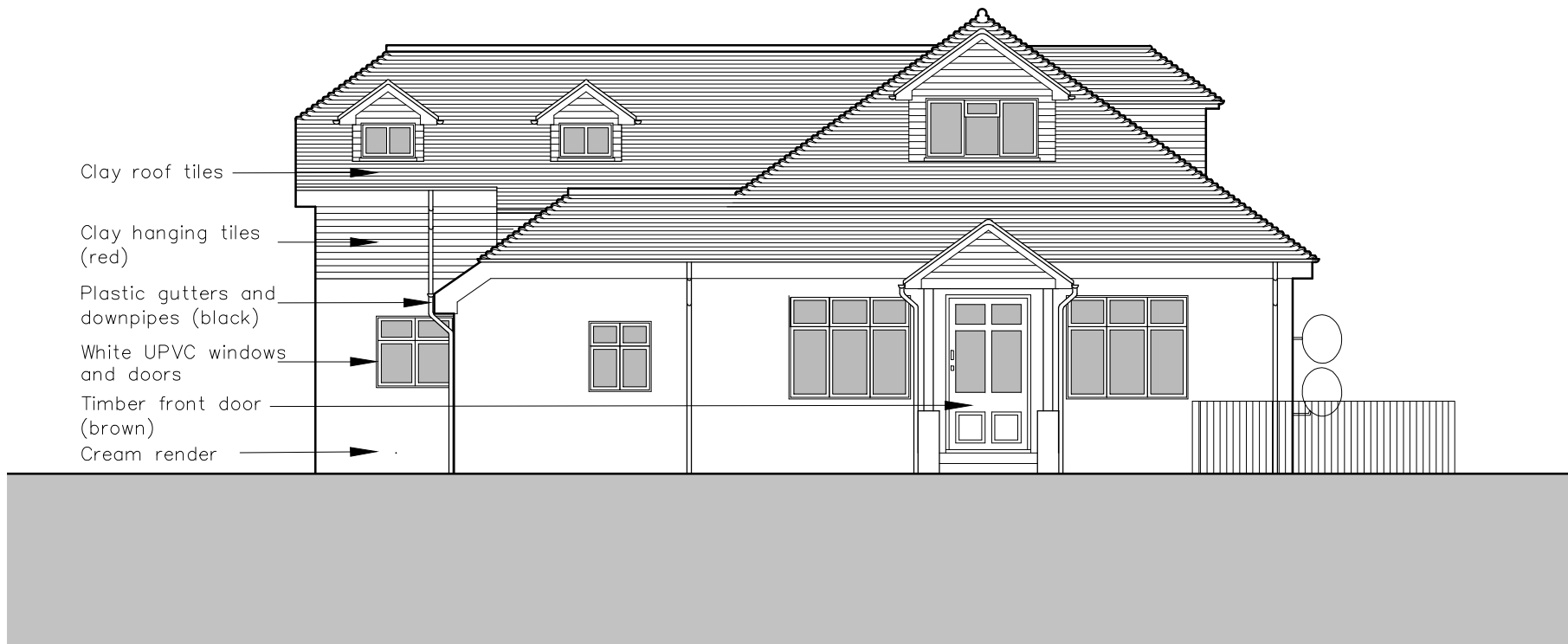
Existing Side (South-West) Elevation 1:100
