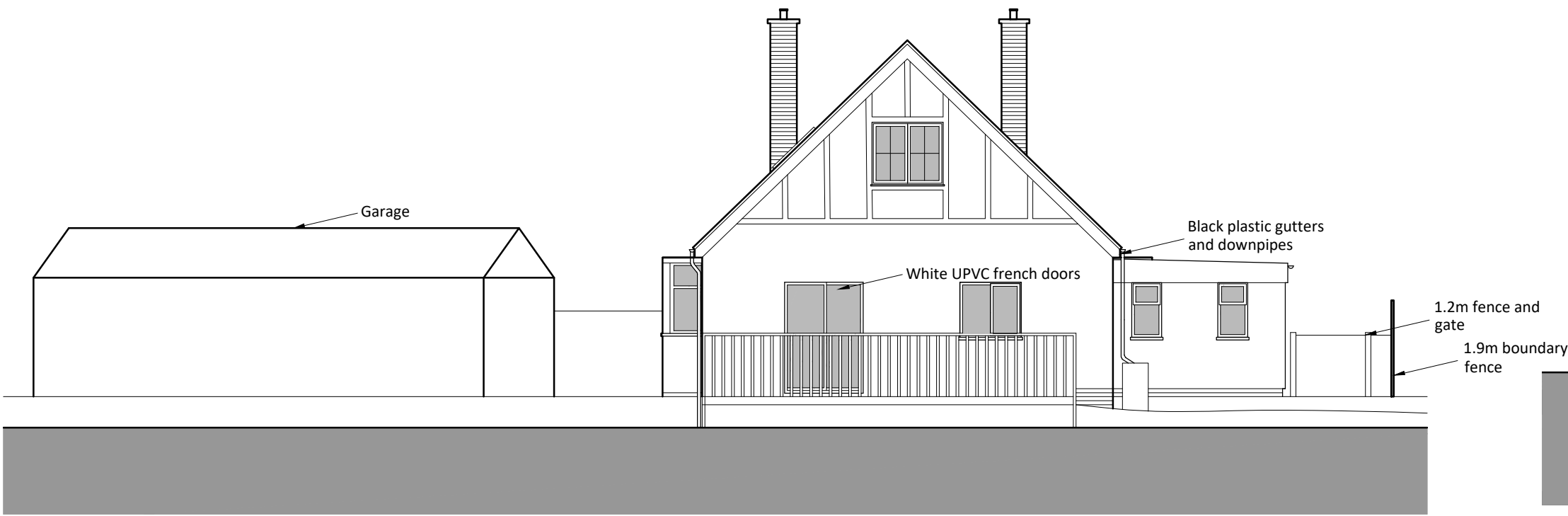
Existing Rear (East) Elevation 1:100
