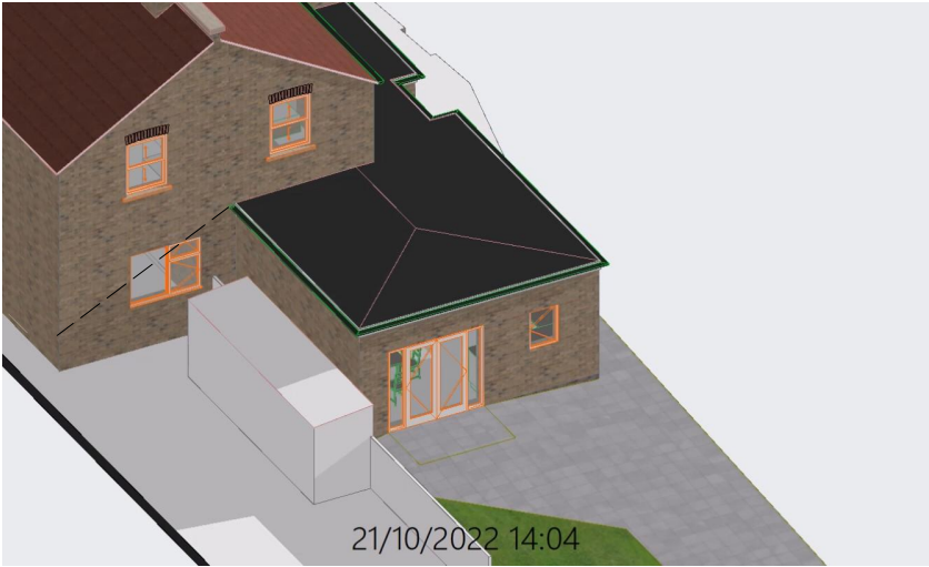
3 March/October equinox 14:00 GMT Sun reaches gable end and proposed extension casts a partial shadow across neighbouring window from 2pm approximately
