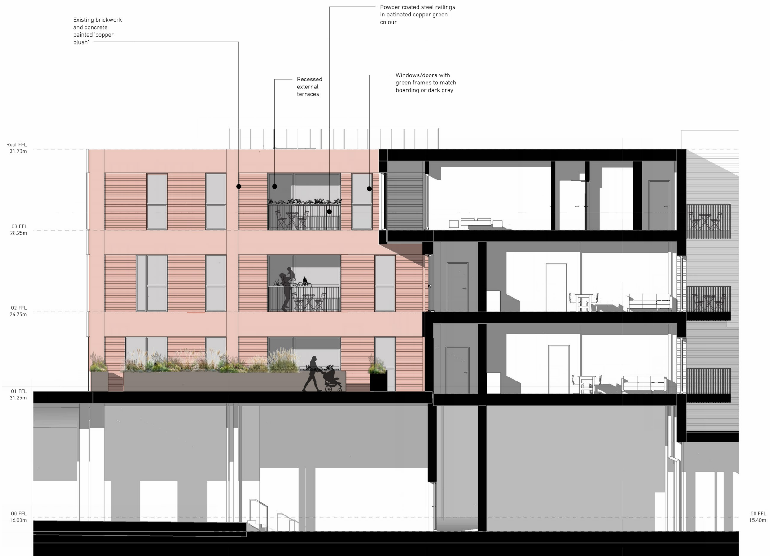
3 Elevation J Mid & Rear Block 1 : 100
