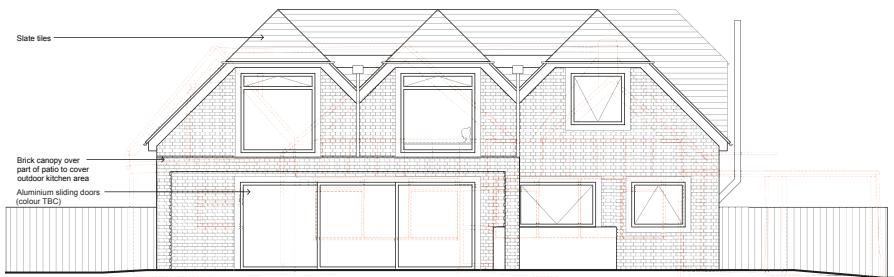
Fig. 22 - Proposed South West Elevation (Pre-app)
