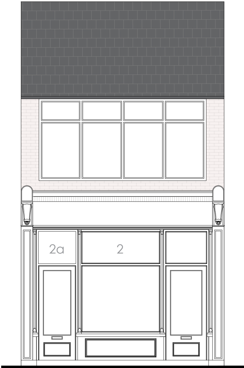
Proposed Front Elevation - Shop front 1:50
