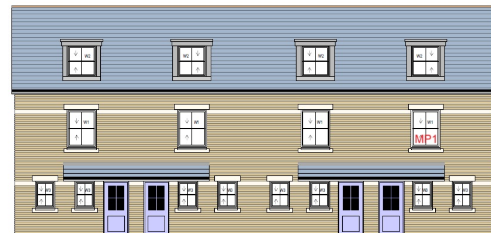
Figure 2: Picture of the Measurement Position & Location on House Elevation (MP1)
