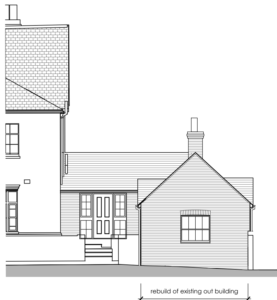
FRONT BUILDING NORTH-EAST ELEVATION Scale 1:100
