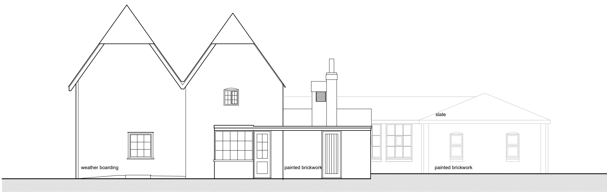
Side Elevation - North Existing scale 1:100 @ A1
