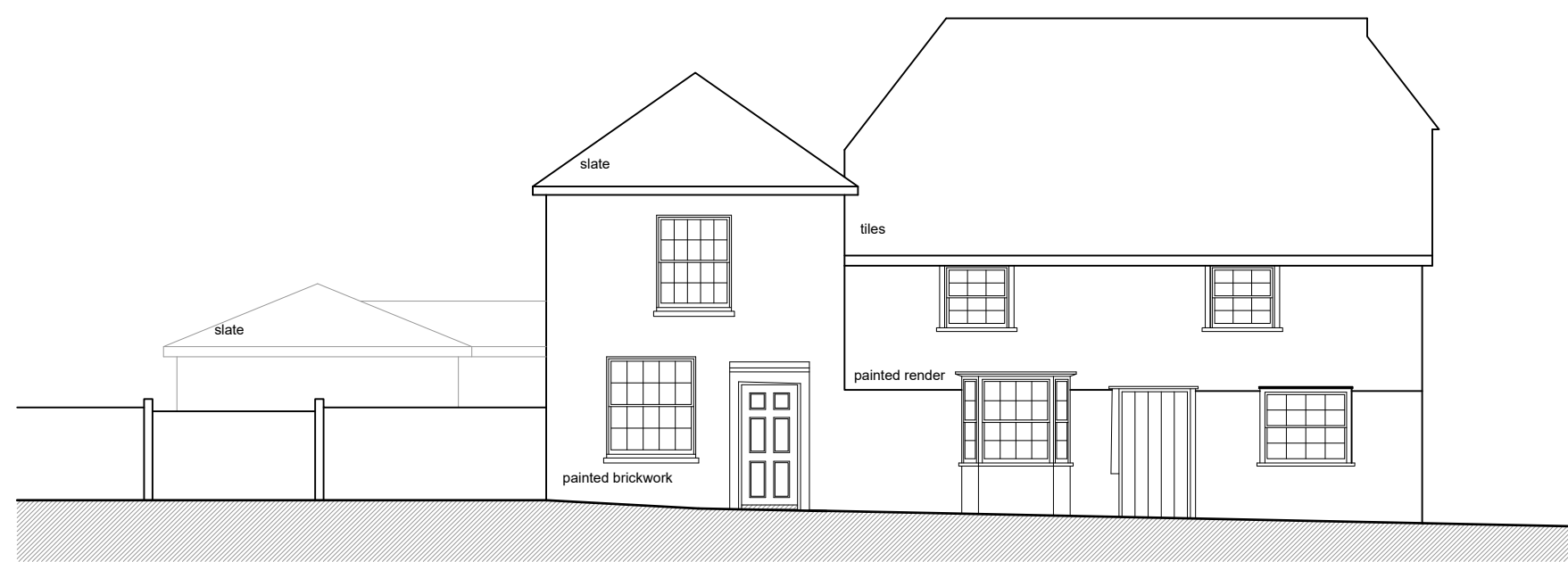
Front Elevation - East Existing scale 1:100 @ A1
