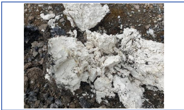
BH201 – Chalk arisings 18.8 to 20m bgl
