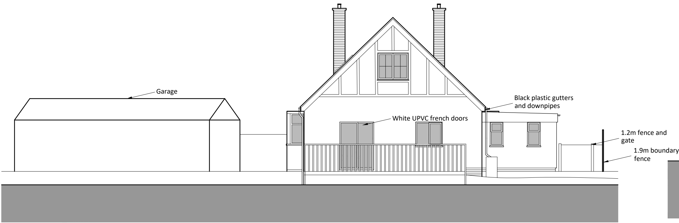
Existing Rear (East) Elevation 1:100
