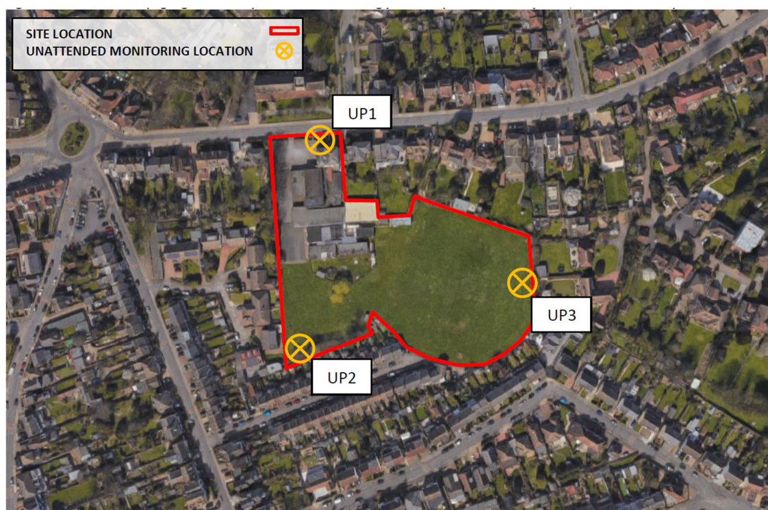
Figure 1: Noise survey measurement positions (ref: 6969_001R_3-0_GC)
