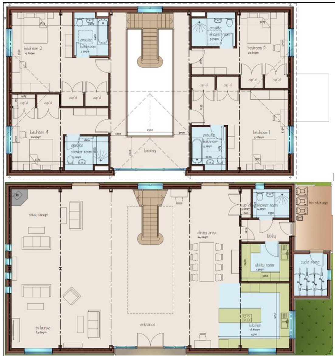
Figure 5. Proposed ground (bottom) and first (top) floor elevations
