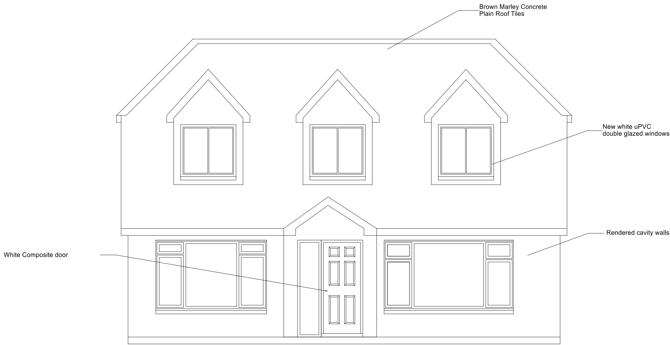
FRONT (EAST) ELEVATION
