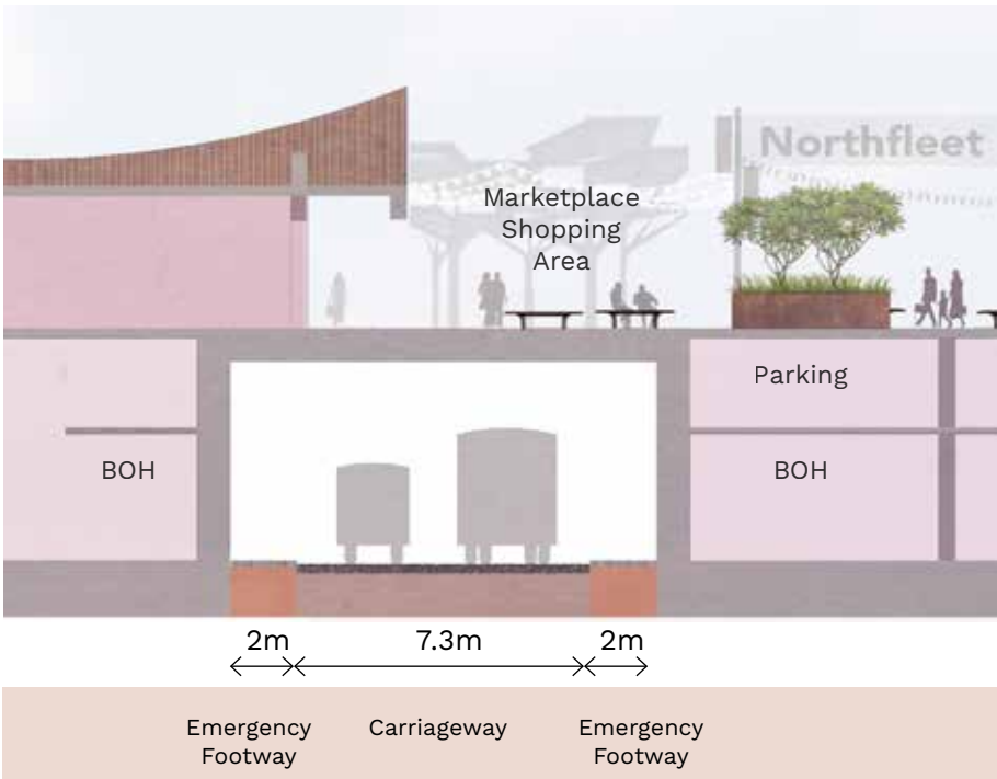
Typical section through the Marketplace podium tunnel
