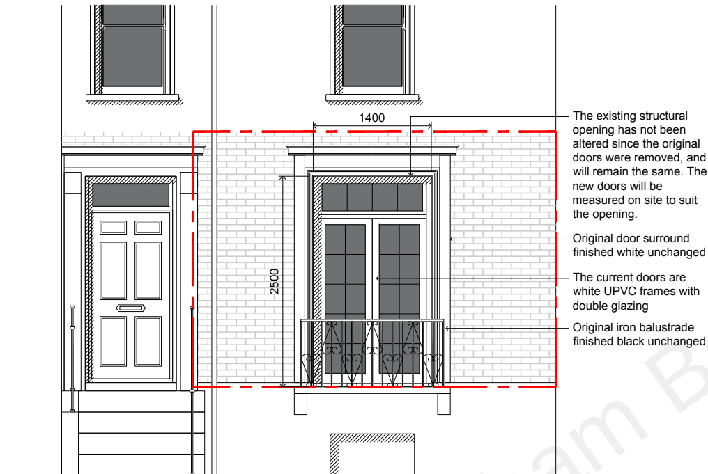
01 | 1:50 | EXISTING FRONT ELEVATION
