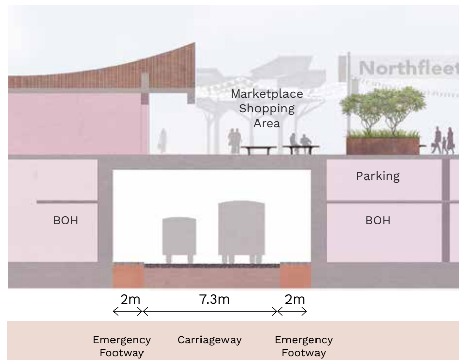
Typical section through the Marketplace podium tunnel
