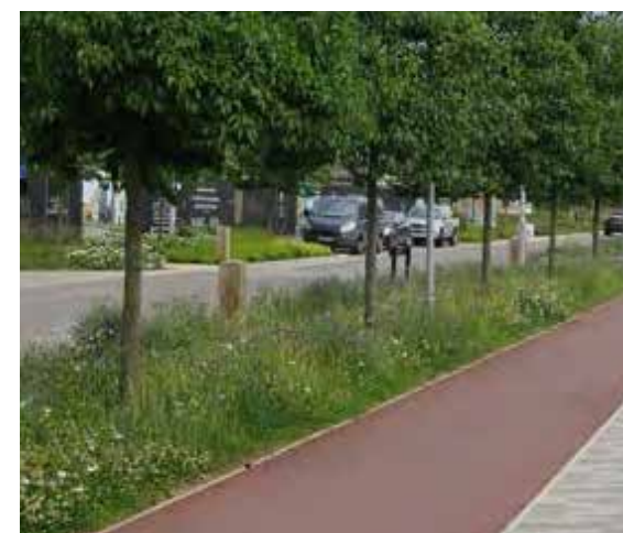
Shallow vegetated swales provide habitat diversity and topographical changes at a micro scale
