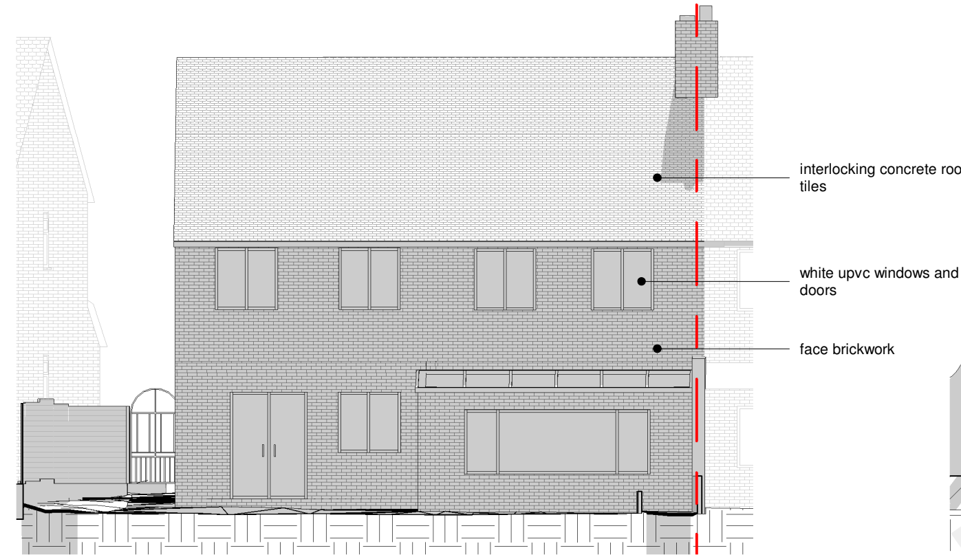
Rear Elevation / Existing
