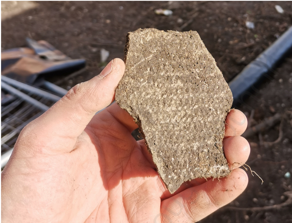
Photo 9: showing PACM from TP03
