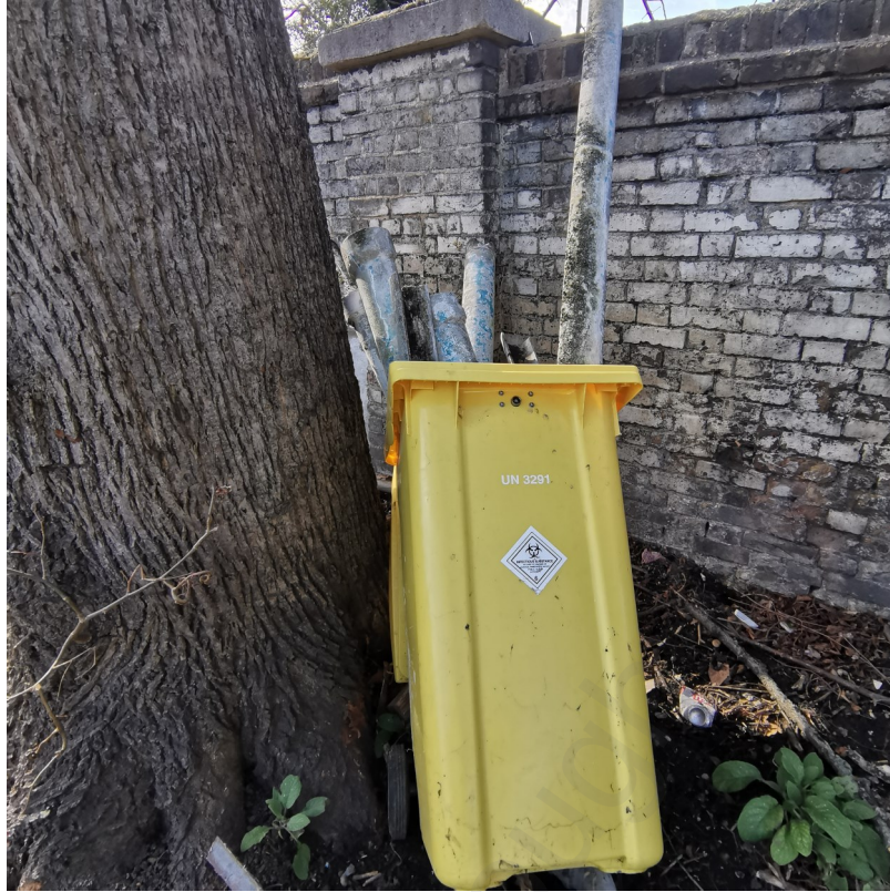
Photo 15: Showing PACMs within (UN Code 6—Infectious Substance Bin)
