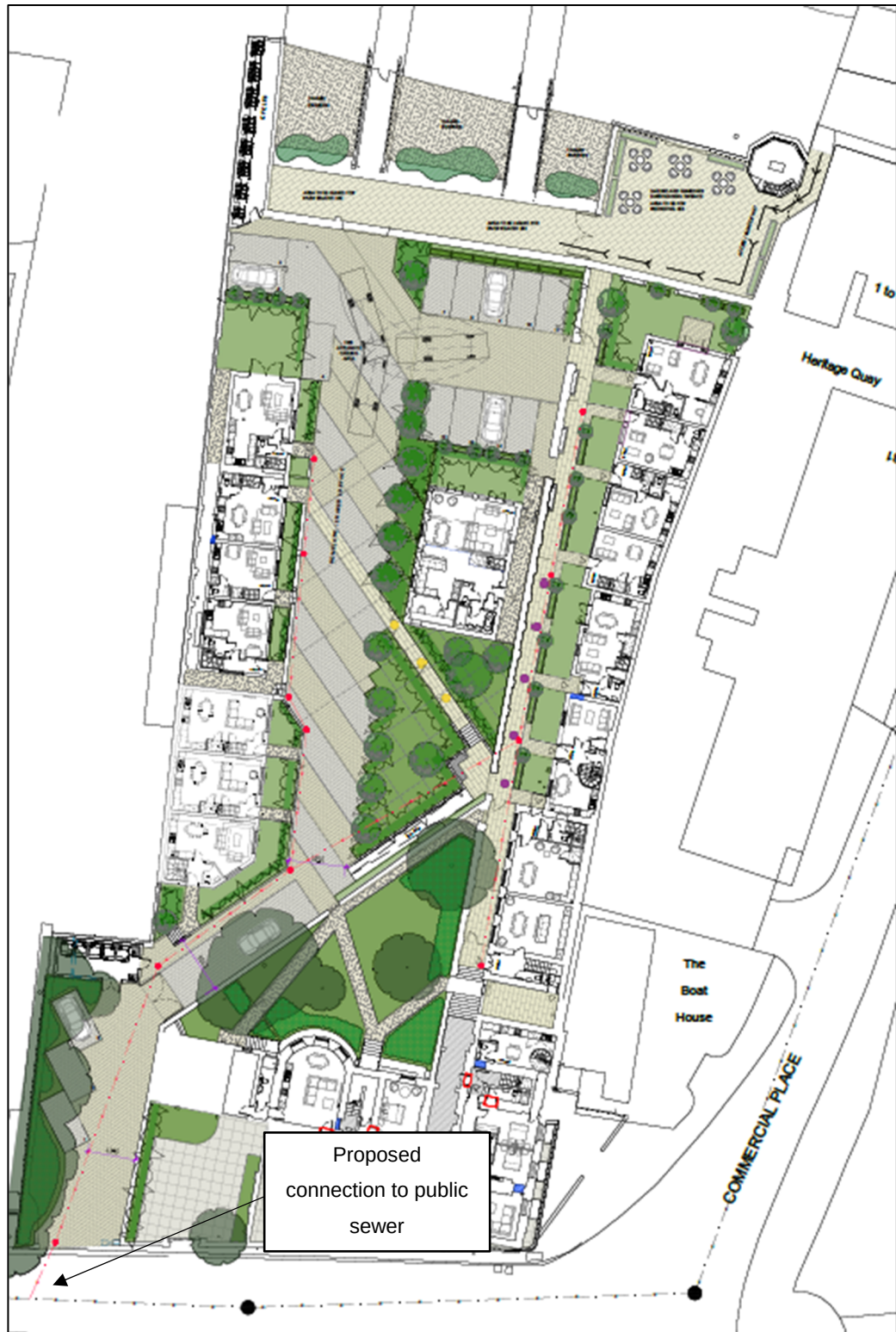
Figure 9.1 – Proposed connection to foul sewer network.
