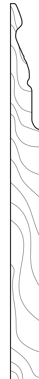
Proposed skirting section Scale 1:2
