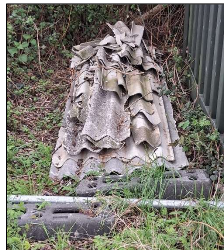
Photo 28: Pile of suspected Asbestos bound cement roof tiles in the south-west.
