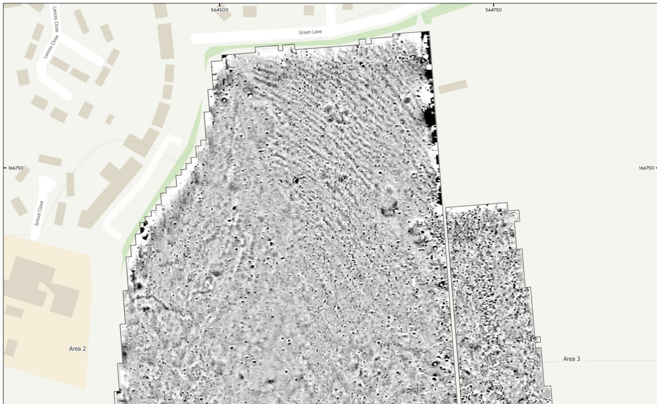
MSTQ2012 - Wrotham Road, Meopham, Kent Figure 8 - Magnetic Gradient (Areas 2 (North) & 3 (North)) 1:1,500 @ A3 © Magnitude Surveys 2025 Contains Ordnance Survey data © Crown Copyright and database right 2025
