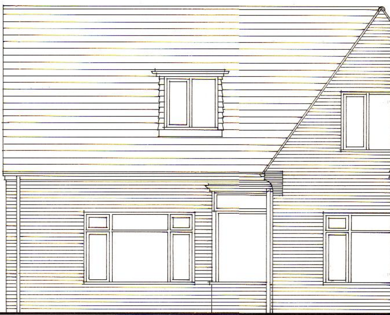
EXISTING FRONT ELEVATION
