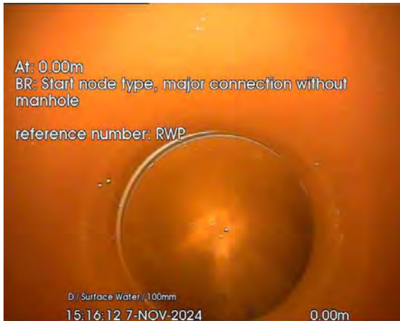
370.jpg, 00:00:02, 0.00 m Start node, major connection without manhole, reference: RWP
